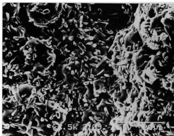
図 2 Surface of SA treated titanium ( $\times 1,500$ )
